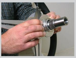
The 'quick grip and rip' system on this new billet hub adapter kit allows you to remove your wheel and hub assembly quickly to get in and out of your vehicle.
