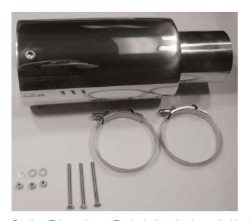
Each muffler is accompanied by two band clamps and three T-head  $\frac{1}{4}$ -20 x 3" cap screws with nuts and washers. CAUTION: This muffler is intended to mount flush on the flat surface of the boat transom. This muffler weighs approximately 12 pounds.
