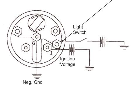
4. Reconnect battery ground. If meter does not read up scale, reverse meter leads.
