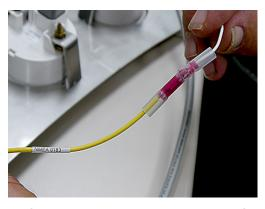
6. Connect white wire (NEMA 0183 Output) pre-terminated with butt connector to yellow wire (NMEA 0183 Input).
