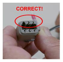
5. Install red power wire in pin location 1 or 6. Install black ground wire in pin location 2 or 5. Visually inspect wire pin for proper installation. Reinstall wedge lock and weather gasket. Reinstall connector to gauge.
