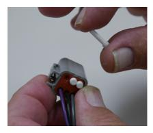
3. Using small screw driver remove wedge lock from connector.
