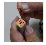
1. Remove 6 pin Deutsch by depressing release tab and pulling outward.
