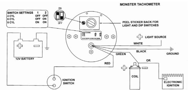
NOTE: This tachometer operates on standard, factory electronic and high-performance electronic racing ignitions, such as Laser II, Hy Fire and MSD. This tachometer is **NOT** recommended for use on Accel BEI or Laser I ignitions.
