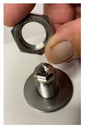
Using a 3/8" Allen wrench, hold the quick pin base and tighten the 1 1/8<sup>th</sup> mounting nut.
