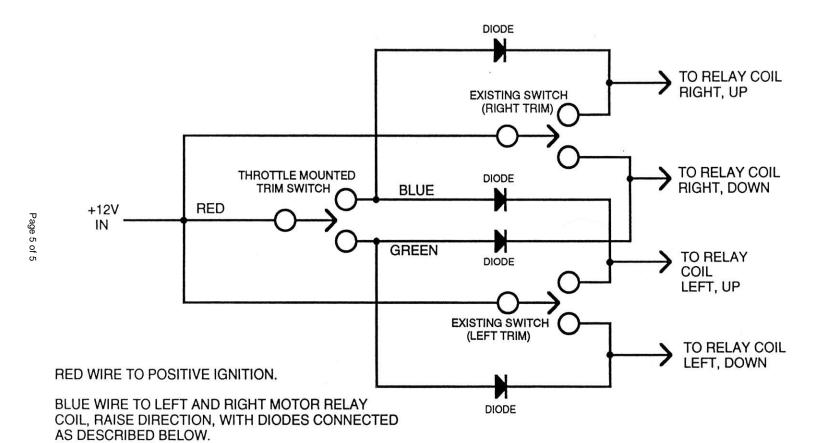
GREEN WIRE TO LEFT AND RIGHT MOTOR RELAY COIL, LOWER DIRECTION, WITH DIODES CONNECTED AS DESCRIBED BELOW.
