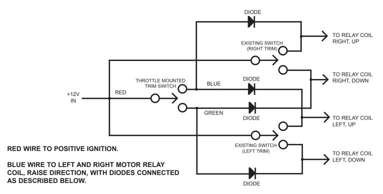
GREEN WIRE TO LEFT AND RIGHT MOTOR RELAY COIL, LOWER DIRECTION, WITH DIODES CONNECTED AS DESCRIBED BELOW.
