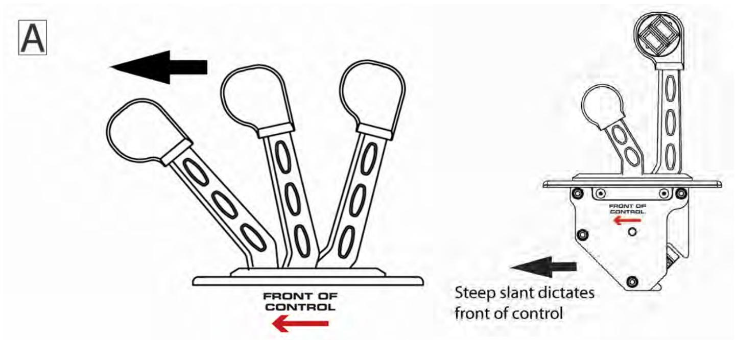
A) Forward cant models; arrow pointing to the ship's bow
