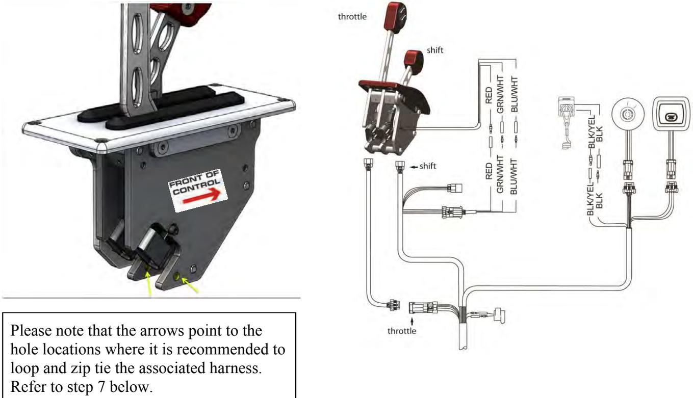
Please note that the arrows point to the hole locations where it is recommended to loop and zip tie the associated harness. Refer to step 7 below.
