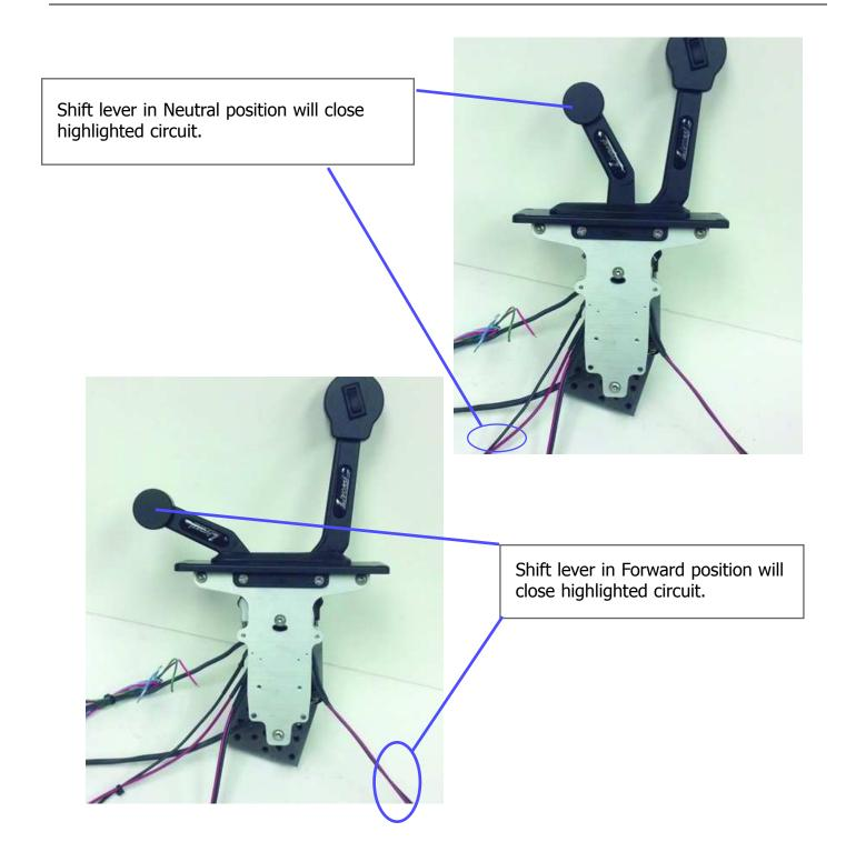
For Livorsi Hybrid Plantinum Series controls where either the throttle is electronic and shift is mechanical or vice versa, the use of 33C series cables are needed.
