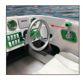
**Control mounts on** starboard side of boat
