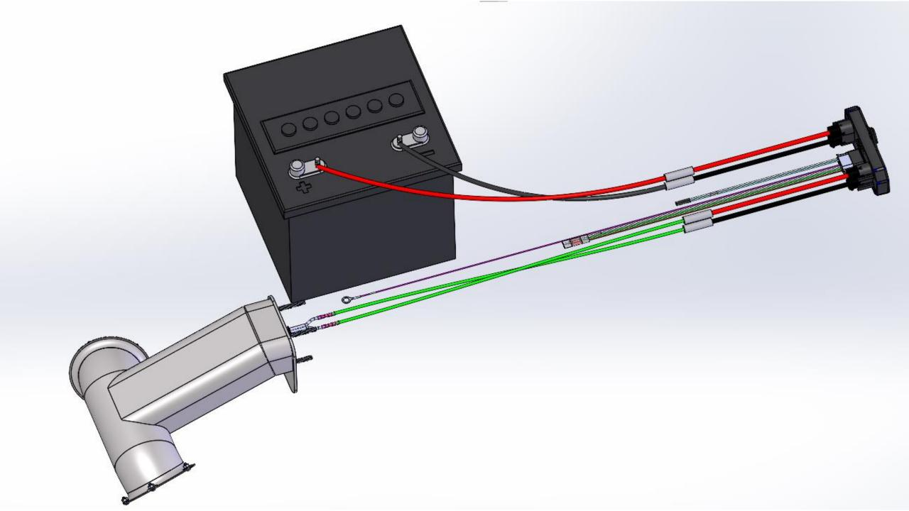
TERMINAL A AND B TO THRUSTER MOTOR WIRES
