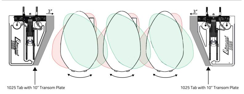
Allow Tabs to be Mounted Outward 3" on Each Side Benefits Include: **Maximizing** Water Cooling & **Minimzing** Prop Aeration
